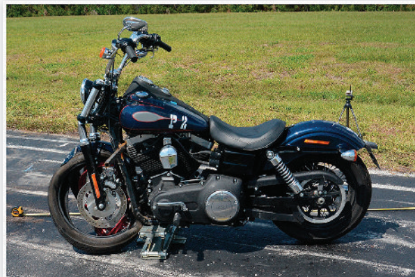
FIGURE 10 Left-side view of M2 showing damage sustained during Test 5, where the wheelbase reduction was 12.8 in.
