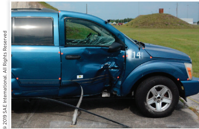
FIGURE 13 Right-side view of C2 showing damage sustained during Test 11, where the maximum crush was 10.3 in.
