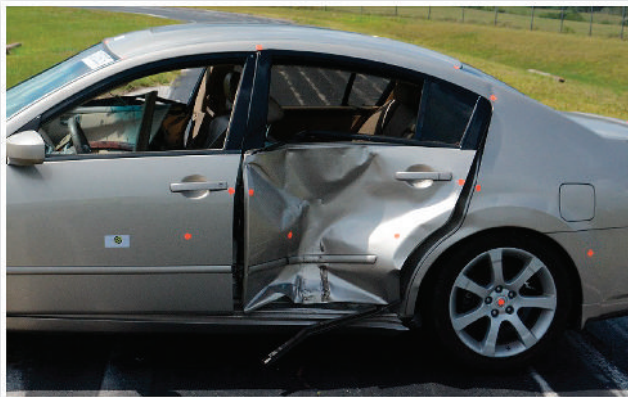
FIGURE 9 Left-side view of C1 showing the impact damage sustained during Test 5, where the maximum crush was 8.6 in.
