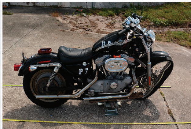
FIGURE 20 Right-side view of M7 showing damage sustained during Test 24, where the documented wheelbase reduction was 8.9 in.
