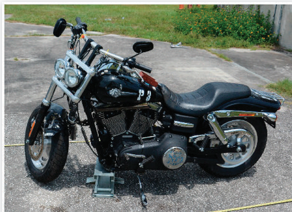
FIGURE 12 Left-side view of M3 showing damage sustained during Test 8, where the documented wheelbase reduction was 3.3 in.
