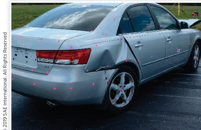
FIGURE 15 Right rear view of C3 showing damage sustained during Test 22, where the maximum crush was 2.1 in.
