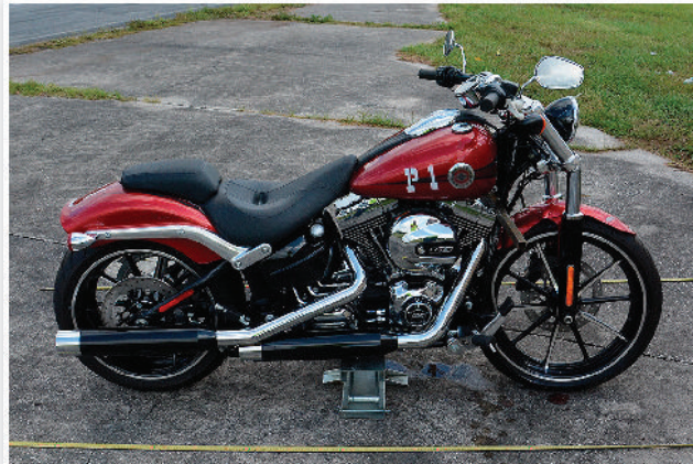
FIGURE 10 Left-side view of M2 showing damage sustained during Test 5, where the wheelbase reduction was 12.8 in.
