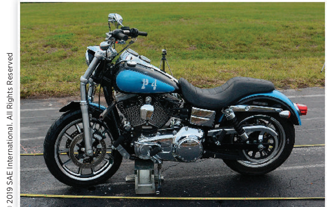
FIGURE 14 Left-side view of M4 showing damage sustained during Test 11, where the documented wheelbase reduction was 10.7 in.
