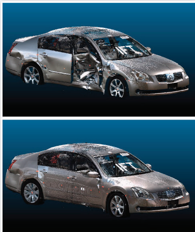
FIGURE 4 Upper image: postimpact 3-D scan data of the 2006 Nissan Maxima (C1). Lower image: compilation of pre- and post-impact scan data, merged using CloudCompare.
