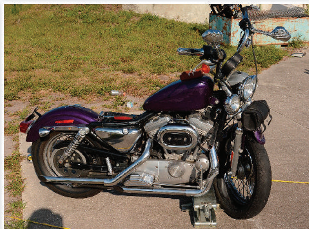
FIGURE 18 Right-side view of M6 showing damage sustained during Test 23, where the documented wheelbase reduction was 8.8 in.
