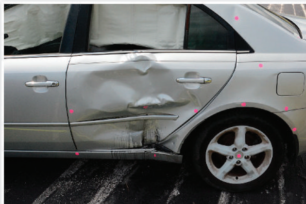
FIGURE 19 Right-side view of C3 showing damage sustained during Test 24, where the maximum crush was 4.2 in.
