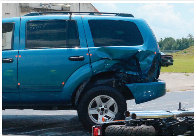
FIGURE 11 Left rear view of C2 showing damage sustained during Test 8, where the maximum crush was 9.1 in.
