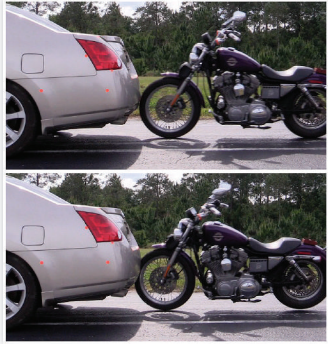
FIGURE 6 Example of low-speed test impact configuration and behavior. Here, first contact and maximum engagement are shown for the 7.1 mph test. Notice the trailing edge of the front fender is contacting the leading portion of the frame and the rear tire is lifted off the ground.
