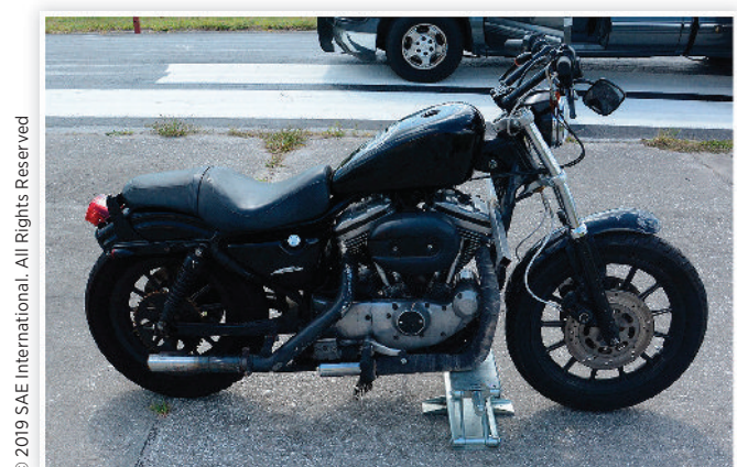
FIGURE 16 Right-side view of M5 showing damage sustained during Test 22, where the documented wheelbase reduction was 4.3 in.
