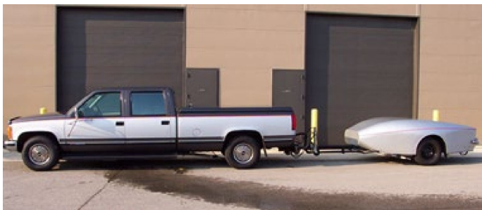
Figure 1 – Skid Trailer used by McIsaac and Garrott
