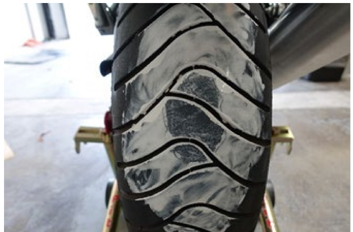
Figure 6 – Paint on Tire After Lowering it Onto the Paper
