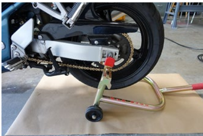
Figure 5 – Rear Wheel of Motorcycle Suspended on Stand Above Paper
